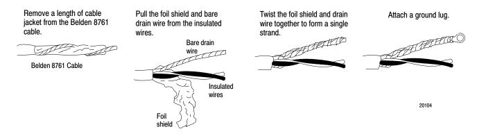
5. Ground the single strand (at the ground lug end) to the grounding stud on the I/O chassis or by using single-point grounding.
