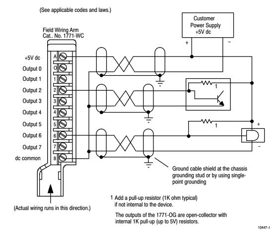
7. Connect TTL output devices using Belden 8761 shielded cable as shown in the connection diagram. Do not exceed 50 cable feet for any output device. Connect the insulated wires to their respective terminals on the field wiring arm.
