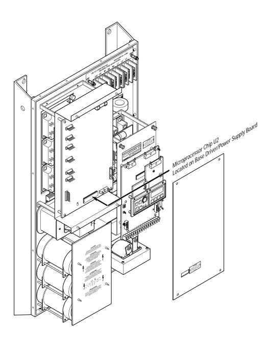
For B075-B125 & C075-C125 ratings, microprocessor chip U2 located on the Base Driver/Power Supply Board has the following firmware identification:
