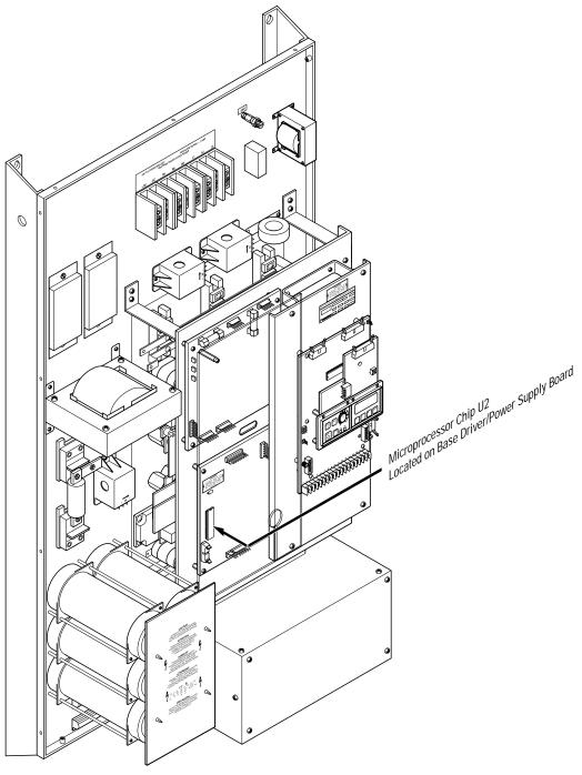
For B150-B200 & C150-C200 ratings, microprocessor chip U2 located on the Base Driver/Power Supply Board has the following firmware identification:
