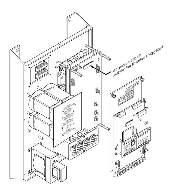
For B040-B050 & C040-C050 ratings, microprocessor chip U2 located on the Base Driver/Power Supply Board has the following firmware identification:
