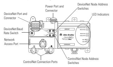
The DeviceNet connection port is located on the top left corner of the device. See the section titled Connect the CN2DN Device to a DeviceNet Network for more information.
