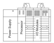
You can configure a system with one, two, or three local chassis, for a maximum total of 30 local I/O or communication modules. You connect multiple local chassis together with chassis interconnect cables to extend the backplane signal lines from one chassis to another.
