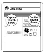
**2.** Loosen the captive carrier retaining screw and swing the carrier door open.
