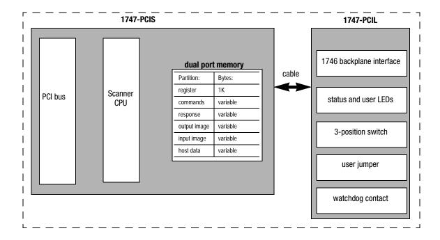
The dual port is an 8K byte memory partition (optionally battery-backed) that provides an interface between the integrated scanner and your application software that resides on the host.
