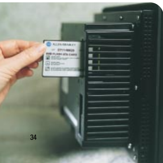
PanelView 300 – 1400 terminals support ATA Memory Card usage.
