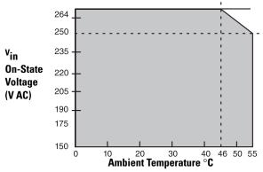
The area within the curve represents the safe operating range for the module under various conditions of user supplied 220V AC supply voltages and ambient temperatures.
