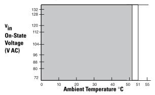
The area within the curve represents the safe operating range for the module under various conditions of user supplied 220V AC supply voltages and ambient temperatures.
