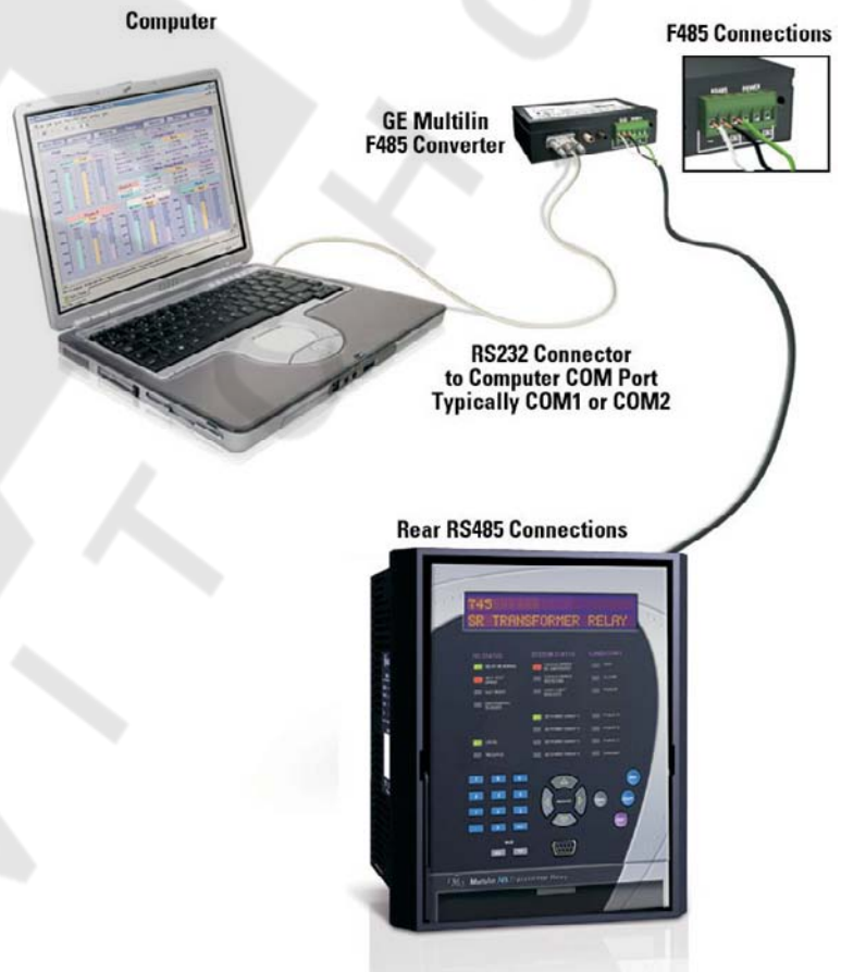
FIGURE 4-3: Communications using rear RS485 port
