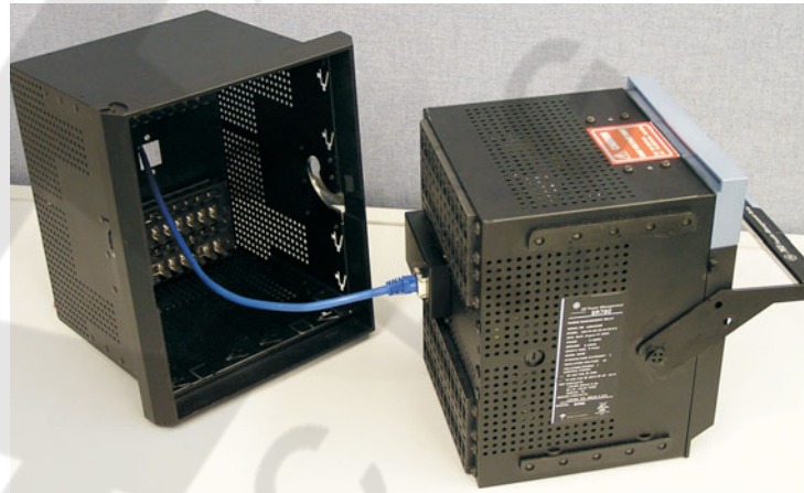
FIGURE 3-9: Ethernet cable connection
