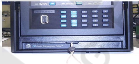
FIGURE 3-8: Drawout unit seal
