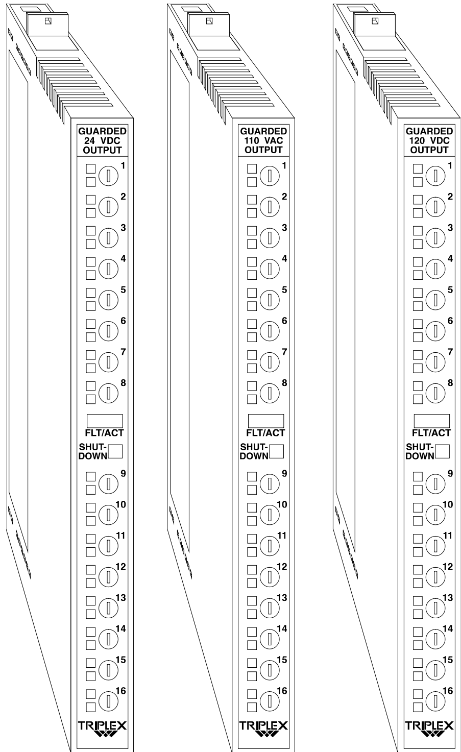
Figure 2. Monitored Guarded Output Modules.
