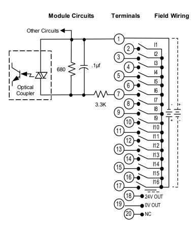
Note: If the 24V OUT pin is used to connect to input devices in the field, the isolation specification for this module changes to:
