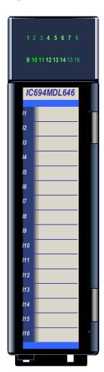
The **24VDC Positive/Negative Logic 16 Point Input** module, IC694MDL646, provides 16 input points in one group with a common power input terminal. *The on and off response times for this module are typically 1 ms.* This input module can be wired for either positive logic or negative logic. Input characteristics are compatible with a wide range of input devices, such as pushbuttons, limit switches, and electronic proximity switches. Current into an input point results in a
